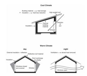
\* Insulation - material used for building which prevents heat passing through it
